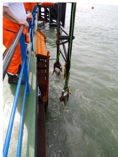
Dual Echoscope® systems deployed from a single mounting frame
